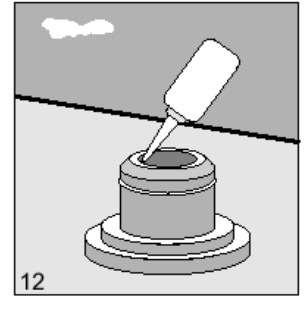
Coat the inside of the gasket, near the O-rings, with petroleum jelly
